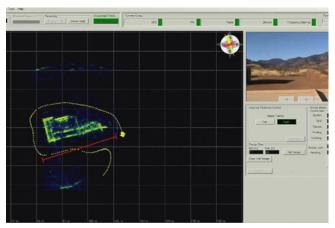
O-PEN system mounted on HMMWV and Image of building complex created by the O-PEN radar system during a drive-by at a desert site.
