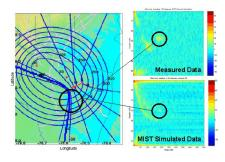
BELOW: SIGINT Collector Modeling - MIST outputs time-domain sampled data that can be processed to produce a "spectrum analyzer" or "oscilloscope" display, and evaluate time difference of arrival, or specific emitter identification processing techniques.
