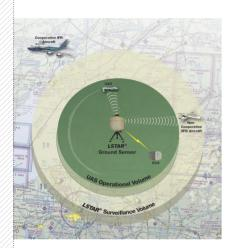
Sense-and-avoid (SAA) technology is essential to enabling flights beyond the line of sight of the operator. One example of SAA is SRC's GBSAA radar system. It was developed for the U.S. Army to allow UAS to operate in the National Airspace System without a chase plane or a ground observer. It uses LSTAR® ground sensors to detect airborne traffic, providing the UAS operator with the information necessary to maintain separation between their UAS and other airborne traffic.
